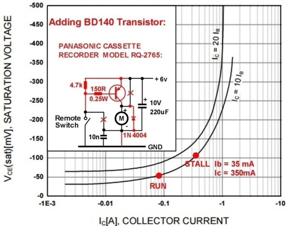
As the graph above shows it is quite easy to get the BD140 transistor into heavy saturation for collector currents of 350mA or below with 35mA of base current. This means that even for the motor in the stalled condition, the voltage drop across the transistor is close to only 100mV. This is far superior to the series 6.8R resistor idea that drops 2.4V.
