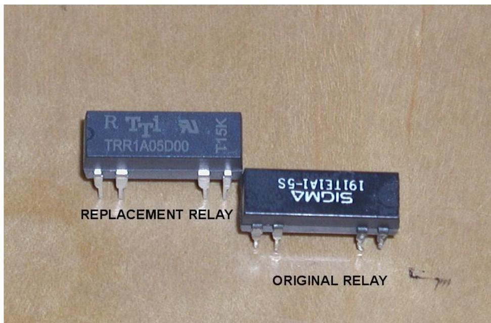
PT made a modification to the Sol-20, by adding 6.8R resistors in series with the relay's contacts, the explanation being to prevent the relay contacts becoming welded together. My Sol-20 did not have these resistors fitted.
