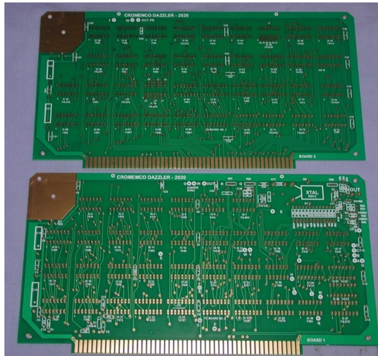
Cromemco Dazzler replica pcb's unpopulated.
