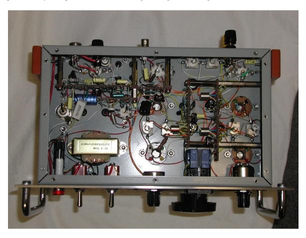
The Chassis is machinery grey painted steel. The tube sockets are ceramic. The adjustment points/trimmers all project to the chassis top for easy alignment.
