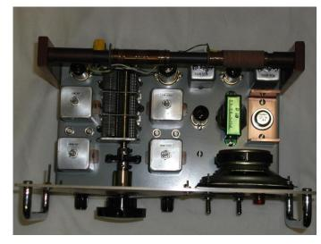
The 23:1 ratio matching transformer was a genuine part made by Beacon Radio in NZ in the early 1960's. The aluminium clamp was anodised green later in the mid 1970's. The IF transformers are American Miller units. The coils in the larger cans were custom designed using high permeability mil spec cores and discarding the original windings.
