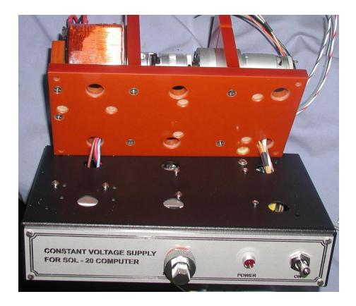
The recessed holes in the top insulating panel allow for the seven screw heads projecting from the chassis surface, one of which is the Earth stud.
