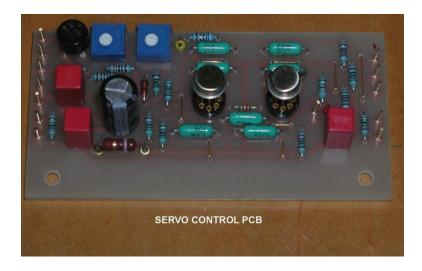
The pcb tracks were drawn in Microsoft Picture IT, laser printed to an iron on pcb film and the board etched with Ferric Chloride. The interesting pale green high quality 0.1uF axial ceramic capacitors were made by the Corning Glass Works.
