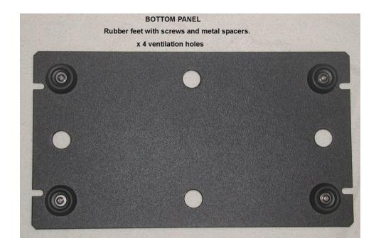
When rubber feet are fitted it pays to use metal spacers so that the rubber is not excessively compressed and the screws can be tightened up so that they don't come loose later. Also, stick on rubber feet as an option are a waste of time as the glue fails and they fall off, so don't be tempted to use them, even though it appears to save you time and it appears to be a plausible idea.
