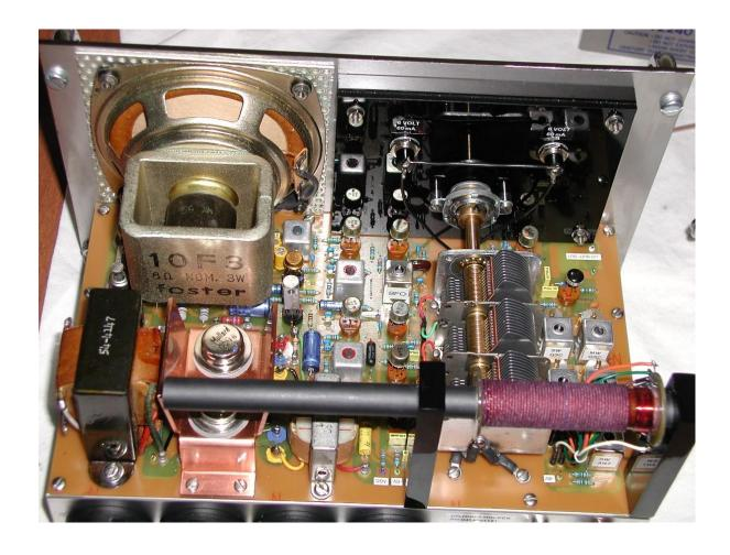
The 4 panel mount battery holders are just visible on the lower edge of the picture each contain two C cells. The performance of this type of radio is practically identical to a communications radio like the Eddystone EC-10, except for the higher power 4 watt audio output stage.
