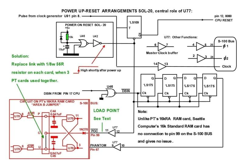
Looking at "Area B" of the PT 16KRA ram cards, this area jumper is to set if the memory is operating in *protected* or *unprotected* mode and how it might behave when power is initially applied or restored after a power failure. I'm not sure of the application of this as Ram is "Forgettory" and after a power failure has lost its data, unless they are referring to what might happen after a short (transient) power glitch or very brief power supply dropout.
