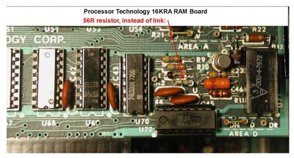
I would therefore recommend that if three 16KRA processor technology ram boards are used in the same Sol-20, and especially if another card is used that connects to pin 99 of the S-100 bus, that 56R resistors are used instead of wire links in the Area B jumper option of the 16KRA ram board.
