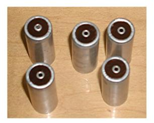
Then there is the issue of replacing the end of the capacitor which was cut off. A convenient choice is fibreglass pcb material. It is easily cut into discs using a 22mm diameter hole saw on the drill press. Then I make a 1/8" central hole and attach a screw & nut to secure it and rotate it, to machine the perimeter down to 16.8mm to be a close fit inside the end of the metal
