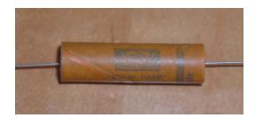
The photo bellows shows some (not all) of the Moulded Silver Mica types which were replaced with new high quality resin dipped silver mica types.
