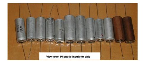
When these capacitors were finished I put a clear surface label on these with the uF value and voltage and the date, to help remind me when they were re-built. Though it is unlikely they will need doing again. (One of these labels can be seen 5<sup>th</sup> from the left in the above photo). Also I decided that having flying leads on the capacitors was a better way to mount them than the original tags that they once had.
