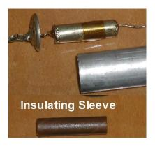
But just one of the four capacitors had a commercial 0.02uF 600V "Dwarf Tiger" capacitor hiding inside it. So I re-built this capacitor and inserted inside the metal canister just as it was before.
