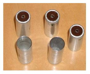
After that I fit 1/8" diameter silver plated brass eyelets in the phenolic end:
