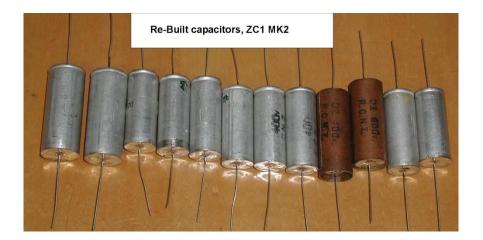
Two of the 0.02uF capacitors have external paper sleeves.
