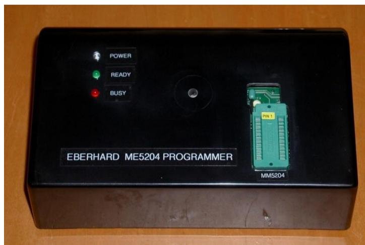
This programmer uses the p + 5p smart over-programming protocol to ensure the MM5204 IC's are properly programmed. It also has a very easy to use interface with excellent hardware, firmware and a very thorough construction and user manual too, all created by Mr. Eberhard.
