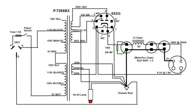
I made use of the centre tap connection on the filament winding to run the power lamp off half voltage. Due to the fact this lamp has a clear glass lens (yes real glass for this one) the filament temperature a yellow-orange color which is easy to see, but not too bright. This way the lamp will likely never require replacing.
