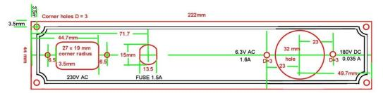
3mm thick engraved silver surface aluminium panel with black ink. 3 mm dia corner holes
