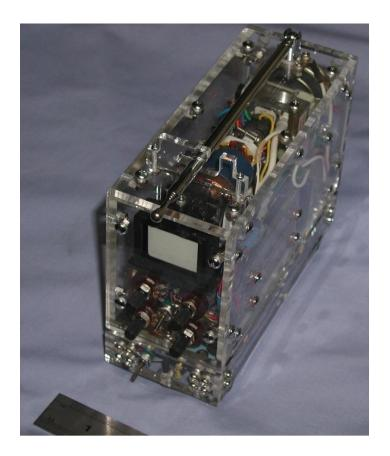
The set is 3.5 inches high x 2.5 inches wide x 6.5 inches long. The battery pack that screws to its base adds another 1.5 inches height including the rubber feet.
