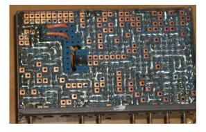
The unit above, in conjunction with the Philips VHF tuner provides a standard video output signal for the "monitor" and the audio to drive the speaker.
