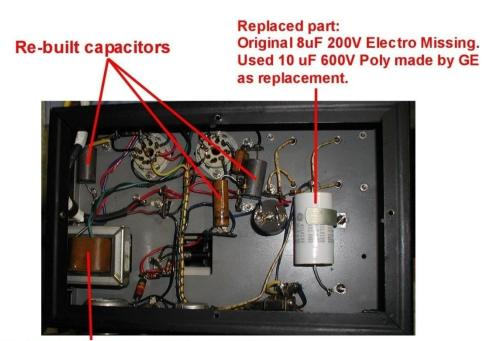
Audio Opt transformer added to avoid high voltages rear panel connectors. 5.5k to 8 Ohm.
