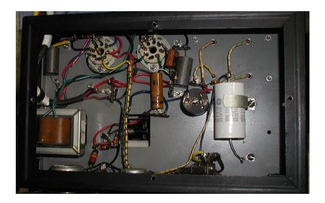
It is important when you fit the audio output transformer to connect one side of the voice coil winding to ground, or otherwise it is still possible to receive a shock from the speaker connections if there are issues with the output transformer's insulation.
