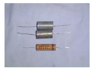
All the resistors and moulded mica capacitors were checked, none were found to be defective so they were left initially. None were found later to be defective on extended testing of the radio either. Though the micas should remain as suspect, still the originals are working and look good so I have no plans to replace them yet.
