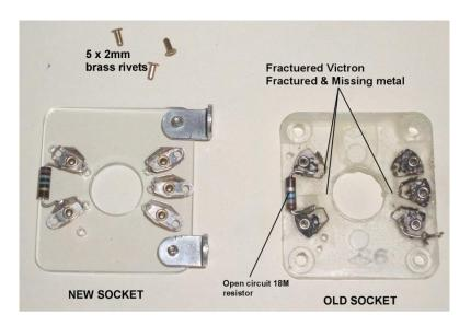
It was unexpected that the 18 Meg Ohm 955 tube's grid resistor was open circuit too. I replaced with a vintage 5% carbon composition resistor. It is important that this resistor does not have any inductive or reactive properties.
