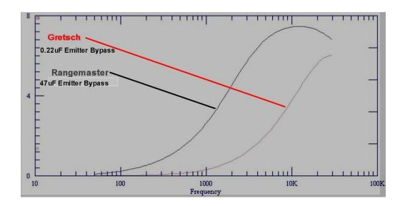
As can be seen due to the large value of emitter bypass capacitor (47uF) in the Rangemaster the frequency spectrum over which it boosts the signal is lower than the Gretsch module all other things equal. Since all of a guitar's fundamental notes lie in the
