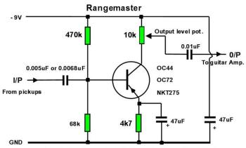
(Note : The ideal transistor is the low noise Germanium AC107)
