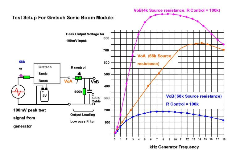
Under this test circumstance (orange graph) the boost unit acts like an attenuator for frequencies under 1000Hz and an amplifier with a gain of about +6 dB per octave with an input frequency above that. The attenuation is fairly heavy at around 100Hz. For example an open low E string is 82Hz.
