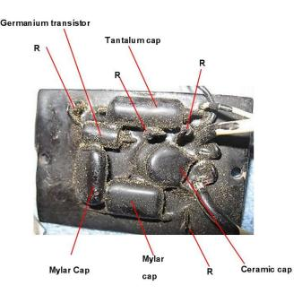
After this module was received it was found that there were in fact two ceramic capacitors, the other one can be seen through the black resin hiding under the one on top of it. Also the axial capacitor turned out to be an Italian made Ducati 15uF 15V, not a Tantalum, but Tantalum is better as it has lower leakage.
