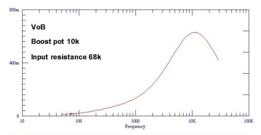
Increasing the boost pot resistance to its max value of 500k drastically lowers the gain and down shifts the overall frequency response:
