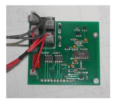
The photo below shows the pcb mounted in the 5153 on existing holes in the metalwork. The hole close to the front is easily tapped with a 4-40 UNC thread, and a screw and nut suffice for the other mounting which is a slot in the metal frame surrounding the monitor's own pcb.
