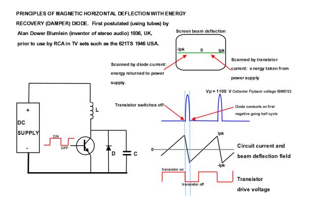
As noted this fundamental design with an energy recovery diode was invented using tubes in 1936 by Mr. Blumlein. He was killed testing Radar equipment in the early 1940's and Winston Churchill described his death as a national tragedy. Pre WW2, the damper diode had not found its way into TV sets in the UK. However, by the post WW2 period the damper diode or efficiency diode or booster diode idea had found its way into TV sets in the USA such as the RCA 621TS model released in 1946.
