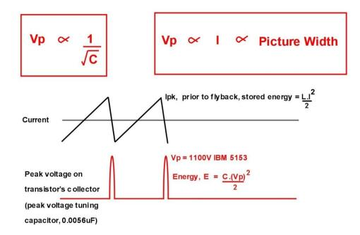
The value of the three series tuning capacitors in the 5153 is about 0.0056uF and there will be some additional capacitance from the transistor and the transformer and yoke windings, probably in the order of about 0.006uF total.
