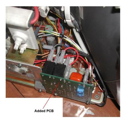
The photo below shows the actual pcb layout, looking from the side of the pcb that faces inwards to the monitor. The high scan rate (EGA) height control and (EGA) H hold control VR1 and VR2 face outwards for easy adjustment. The pcb is 92 x 83mm, the mounting holes 60mm apart an the one near the corner is spaced 5mm from each edge:
