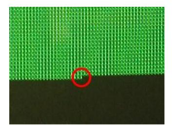
Due to the width of the electron beam and the shadow mask geometry, single green phosphor elements are not the only ones lit, there is a spread around the phosphor trio into the adjacent six green phosphors, making the illuminated pixel less well defined than in a monochrome CRT. Also with tri-color pixel illumination, convergence errors cause a larger spread around what would be the pixel center.
