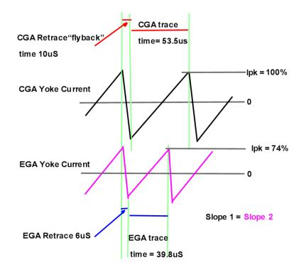
Since the rate of change of horizontal scanning current with time is fixed by the proportions of V/L, of the power supply voltage V and the horizontal output transformer and yoke inductance combination L, the shorter scanning time in EGA mode means that the peak horizontal yoke current lpk, climbs to a smaller value of 74% in EGA vs 100% in CGA scan time.
