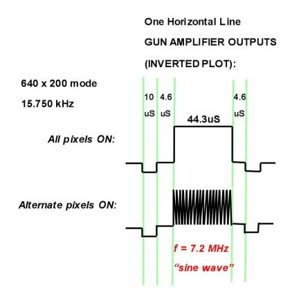
Examining this drive waveform at the gun amplifier outputs (Using a very capable Tek 2465B 400MHz bandwidth scope) the waveform appears sinusoidal, not rectangular and the sinusoidal part has an amplitude of 19V.
