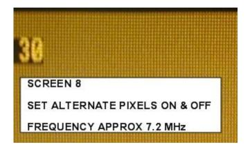
Unfortunately, Color CRT's such as those in the 5153 or 5154 are not generally capable of exactly this sort of resolution. While the phosphor pitch in the CRT from a 5153 or 5154 monitor is small enough to support such a display resolution, the limitations imposed by the CRT's shadow mask and focussed beam diameter are such that a single pixel is not as well defined and the phosphor dots (from phosphor trios of the same color) in the local area are partially illuminated.
