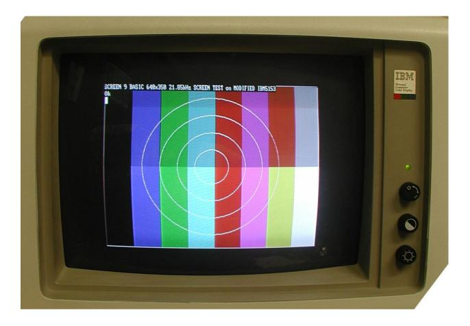
Notice there is a mild degree of Barrel Distortion of the image. The Pincushion correction circuit is a little over zealous running in the high scan rate mode.
