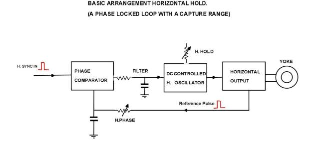
Since the circuit is fundamentally a PLL (phased lock loop) any noise pulses in the H sync pulses are averaged out by the filtering and the horizontal oscillator cannot abruptly respond to sync pulse noise and the line tearing effect eliminated.
