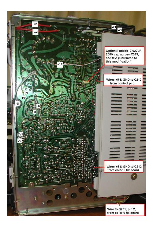
There is a phase error in EGA mode (horizontal picture position offset) that is corrected for by the connections P1 and P2. (see section 6 on how to accurately set set H hold and H phase pots on the main monitor pcb first). This is not often done correctly and the controls H.Hold and H.Phase interact.
