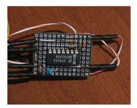
This small color 6 Fix board s simply placed near the cable connector inside some large heat-shrink sleeve and suspended by its own connecting wires. The schematic is shown below:
