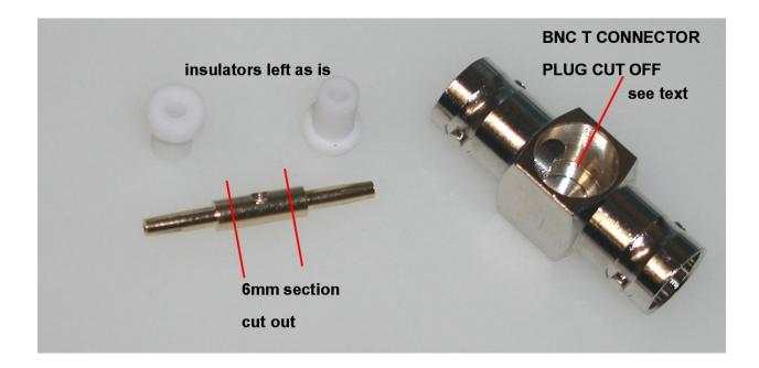
The central pin and insulators are pressed out (they are retained by a small serrated edge press fit washer at one end. A 6mm length is cut out of the central pin area, leaving a 2.0mm base on the socket pin because the central section is exactly 10mm wide.
