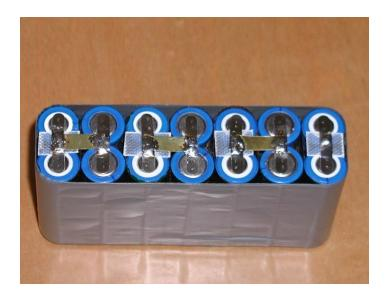
The cells are linked together with 0.15 thick x 5mm wide brass strips as shown. This assembly has the connecting wires added and is covered in fibreglass tape:
