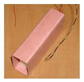
An end cap is placed in one end. The whole case is also varnished to seal the electrical card.
