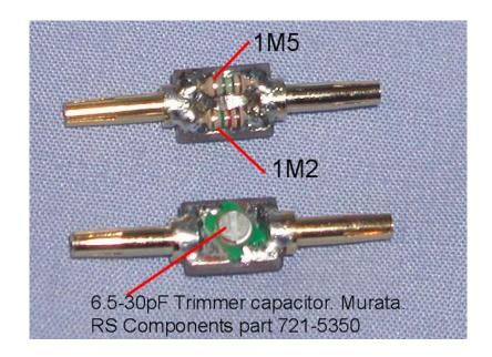
The photo below shows the parts before reassembly:
