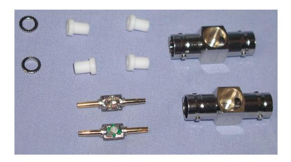
A small piece of tube is used to press in the locking washers and reassemble the connector.
