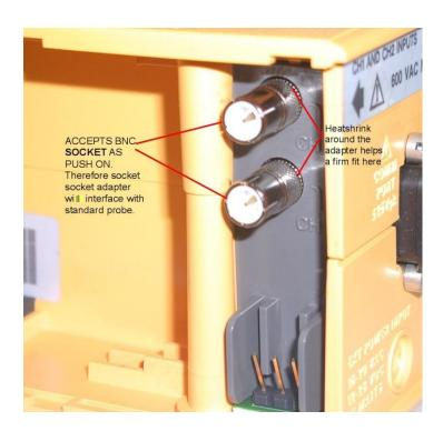
A female – female (BNC socket – socket) adapter now will adapt a standard probe to these fittings. However the 666.6k series resistor and HF compensation capacitor is still required in series. Therefore these can be put inside the socket-socket adapter. This is done by starting with a socket to socket adapter with a T style BNC plug. RS components part number 546-4948. The plug is cut off and just the straight section used. The central hole is bored out just a little to 9mm diameter:
