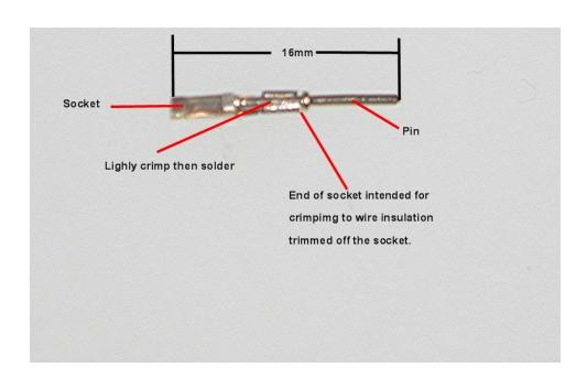
The pin end which is 0.9mm diameter is a tight fit and is inserted into the BNC adapter:
