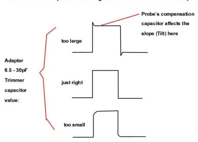
1kHz fast rise square wave signal from 50 Ohm source impedance & x 10 probe:
