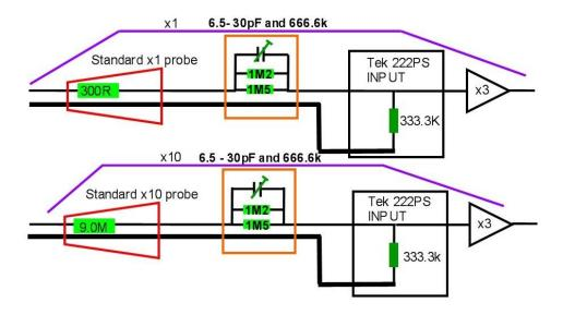
This arrangement ensures that not only do the probes see the correct impedance they were designed for, but the voltage calibration is correct on the scope's display.
