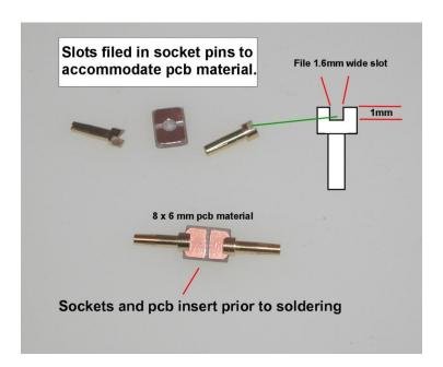
The pins are aligned on the pcb and spun in a drill chuck or lathe to ensure they are on the same axis. After that the assembly is soldered together and the resistors added on one side and the trimmer capacitor on the other:
