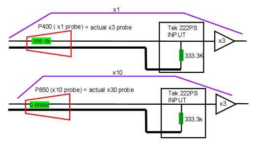
Tek 222PS scope has a 333.3k input resistance unlike most scopes which have a 1M input resistance.
