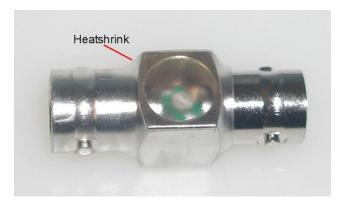
The following photo shows these adapters pushed on to the BNC adapters that were fitted to the 222ps probe sockets. A small amount of plastic is remove from the battery compartment cover to accommodate the lower adapter.
