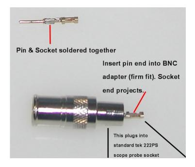
A single piece of heat-shrink sleeve around the right hand half of this adapter also helps make an interference fit with the plastic socket hole in the 222ps probe socket area. The photo below shows these adapters plugged into the side of the standard 222ps probe socket area:
