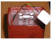
The pcb panel is glued over another layer of card with 24 hr epoxy resin. The connector had unusual pin spacing at 4mm. So a connector body was crafted from some white Bramite (similar to Garolite) and Jaycar 0.9mm socket pins fitted inside it. The external dimensions are 34 x 55 x 125mm.
