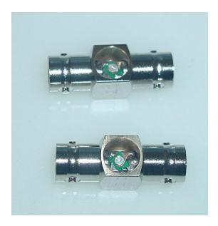
Some heat shrink sleeve is placed over the connector to keep out dust and a small hole can be made in it to adjust the capacitor.
