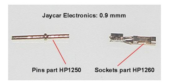
These are crimped and soldered together:
