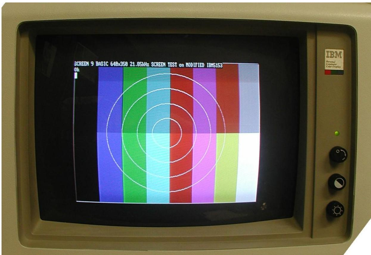
Notice there is a mild degree of Barrel Distortion of the image. The Pincushion correction circuit is a little over zealous running in the high scan rate mode.
