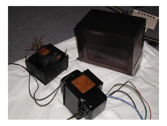
The original POWER transformer (shown in photo upper left above) is not a safe proposition to run again especially here in Australia with our 50Hz supply frequency. The transformer has very aged and cracked insulation and runs an excessive magnetization current on 50Hz.
