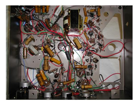
The underside of the chassis is re-wired, all new resistors, wiring and tube sockets. The resistors are now all 2 watt metal film, but yet the same size as the original 1/4 or 1/2 watt types. 500V Silver mica caps were used to replace the original molded micas, and the wax paper caps re-built with poly's with twice the voltage rating.
