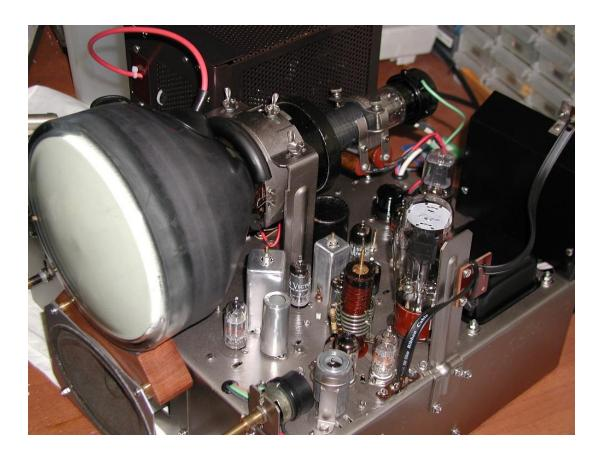
Shown in the photo below is the original power transformer. I took the copper flux band from it and the restored covers off it and added them to a new Hammond 300BX transformer and discarded the Hammond covers which are quite different. The two transformers have very close to the same geometry stack, with the holes placed only a little differently.
