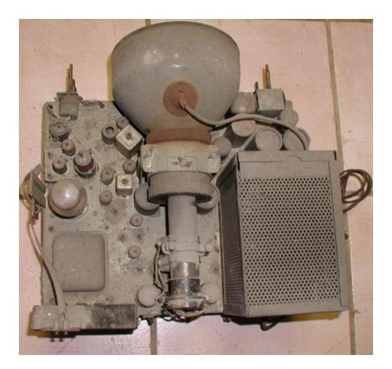
It became standard practice in the post war period to enclose the line output transformer and EHT rectifier in a separate cage, shown on the lower right of the chassis. The Power transformer, lower left was mounted on the chassis under surface to keep it as far as possible from the CRT to avoid the effect of magnetic interference with the beam.
