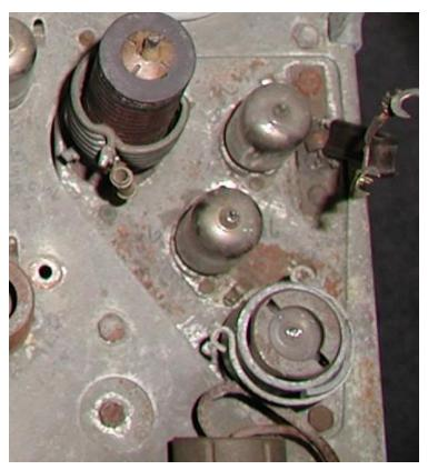
The photo immediately above shows the Tuner area. One of the tubes has a Lead shield with a spring clip holding it in place.
