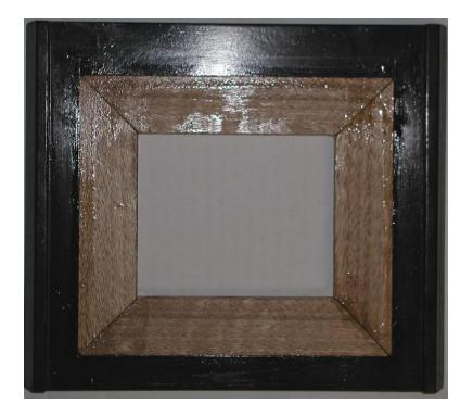
This was then varnished shaped to match the original design and fit the curved CRT face. Appling varnish initially helps with getting the geometry right as the wood is filed away by hand:
